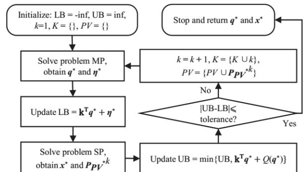
Fig. 2. Solve the TSRB model using C&CG algorithm.
